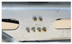
Centralized Grease System Located at Bumper
