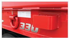
• The standard four strap winches with opposing strap hooks and 4 "D" ring tie downs are conveniently located for efficiently securing the container.
