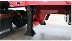
• Jost 2-Speed Crank Down Landing Gear.
