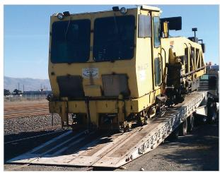
Assist in Loading with the Landoll Standard 12,000 lb. Winch (Choose a 20,000 or 30,000 lb. Winch to Load Totally Disabled Equipment)
