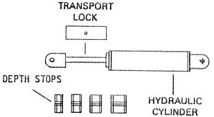
Determine operating depth and use stops accordingly.
