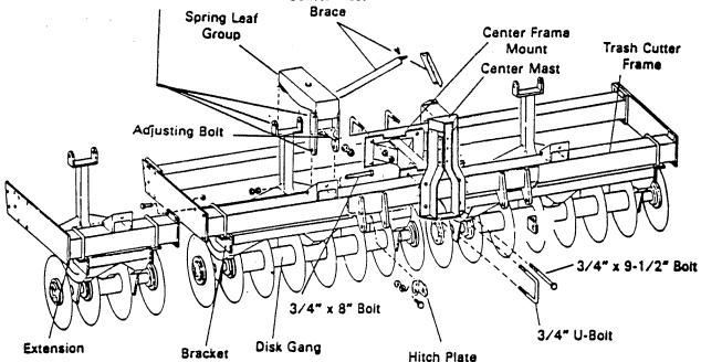
Mount Cat. II and III hitch plate to plate between hitch arms, using  $5/8" \times 1-1/2"$  bolts, lock washers and nuts. Mount one way for Cat. II and turn over for Cat. III.
