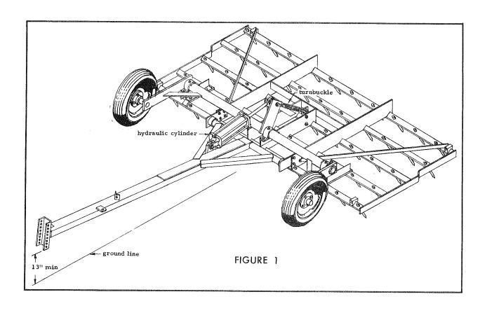
To work properly the harrow drawbar must be a least 13" above the ground surface. To put downward pressure on the rear tooth bar of the harrow the ratchet jack or hydraulic cylinder must be fully extended. The higher the drawbar or hitch point the more pressure can be applied to the rear tooth bar.
