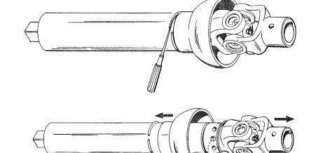
2. Hold assembly over container so that balls will not be lost and slide bell away from joint toward opposite end of tube. If balls do not drop out, slide tube away from joint, forcing balls from cage.
