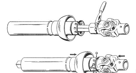
Grease joints, telescoping shafts and guard regularly. This Quick Detachable Free Wheeling Guard is the finest guard built. It is provided for your protection.
