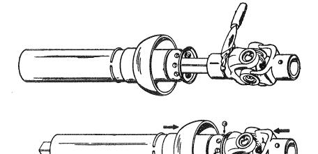
Grease joints, telescoping shafts and guard regularly. This Quick Detachable Free Wheeling Guard is the finest guard built. It is provided for your protection.
