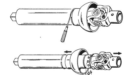
2. Hold assembly over container so that balls will not be lost and slide bell away from joint toward opposite end of tube. If balls do not drop out, slide tube away from joint, forcing balls from cage.
