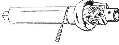
2. Hold assembly over container so that balls will not be lost and slide bell away from joint toward opposite end of tube. If balls do not drop out, slide tube away from joint, forcing balls from cage.
