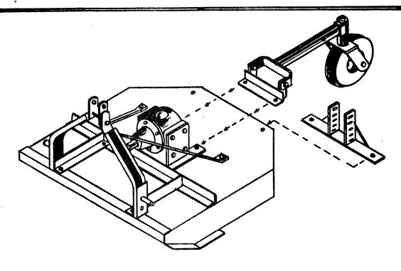
FIGURE 2 Assembly of 3 Pt. Pickup Type Machine
