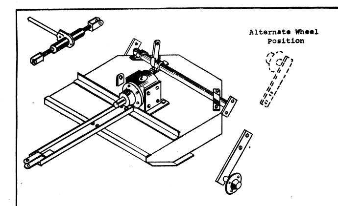
FIGURE 1 Assembly of Drawbar Type Machine
