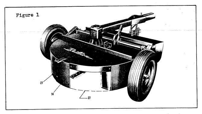
type of material you are cutting will determine the opening to provide for the discharge of the chopped brush.
