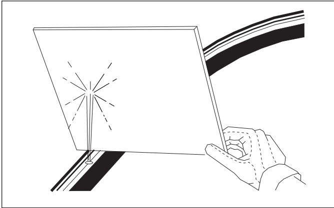
Figure 2-27: Hydraulic Leak Detection
