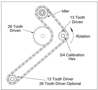
Figure 3-10: Seed Box Calibration
