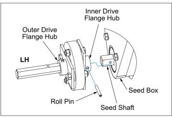
Figure 2-7: Agitator Installation - LH
