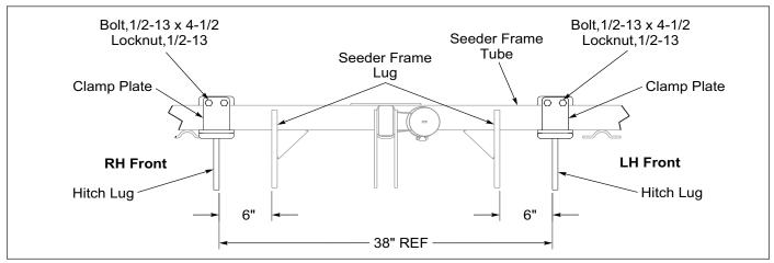
Figure 2-14: Quick Hitch Adapter Kit - Dimensions
