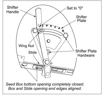
Figure 4-6: Agitator Box Completely Closed.
