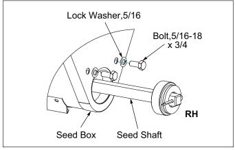
Figure 2-8: Agitator Installation - RH
