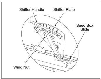
Figure 3-7: Shifter Handle Adjustment
