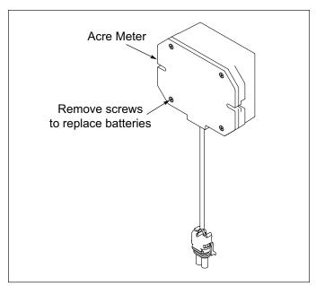
Figure 3-16: Battery Replacement
