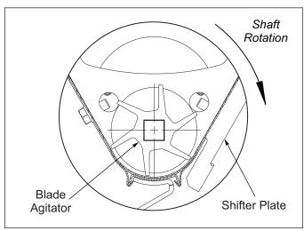
Figure 2-5: Blade Agitator Orientation
