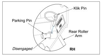
Figure 3-1: Parking Pin Disengaged
