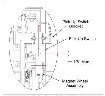
Figure 2-12: Pick-Up Switch Adjustment
