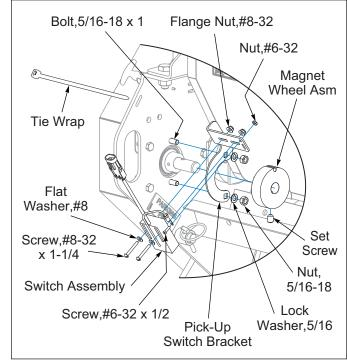
Figure 2-11: Pick-Up Switch Bracket
