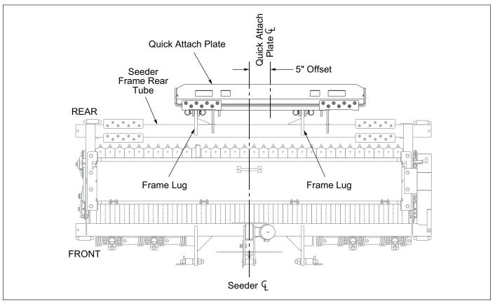
Figure 2-4: Quick Attach Plate Mounted - Offset
