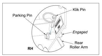
Figure 3-2: Parking Pin Engaged
