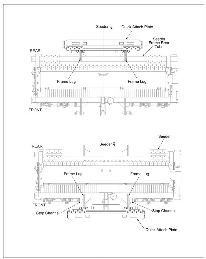
Figure 2-3: Quick Attach Plate Mounted - Centered
