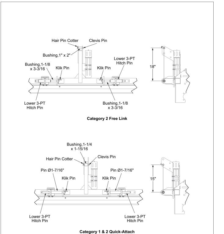
Figure 2-16: Quick Hitch Adapter Kit - Category Pin Positions
