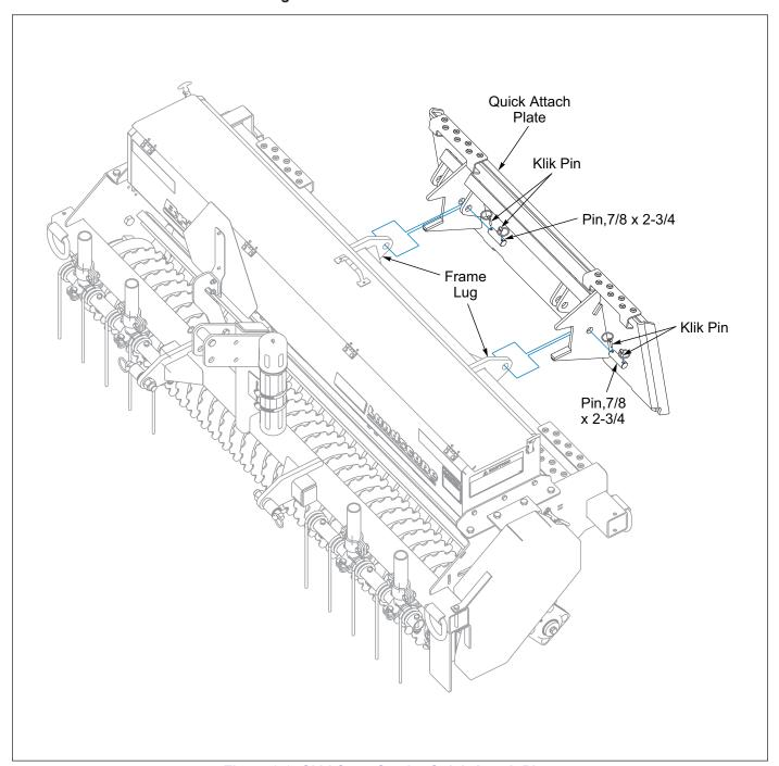
Figure 2-2: Skid Steer Seeder Quick Attach Plate
