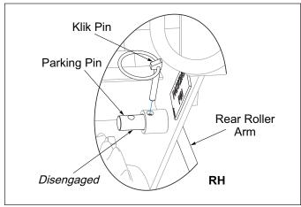
Figure 3-5: Parking Pin Disengaged
