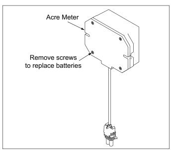
Figure 4-9: Battery Replacement
