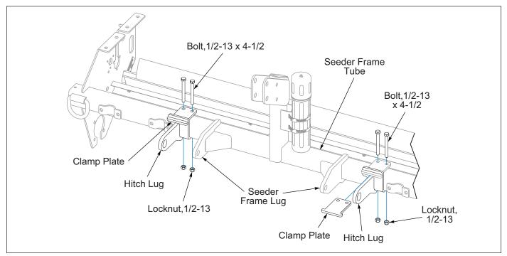
Figure 2-15: Quick Hitch Adapter Kit
