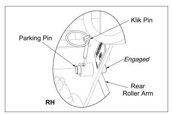
Figure 3-6: Parking Pin Engaged
