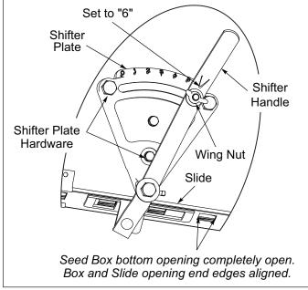
Figure 4-7: Agitator Box Completely Open.
