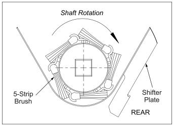
Figure 2-6: Brush Agitator Orientation
