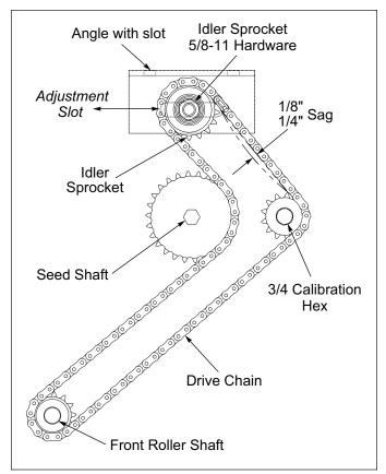
Figure 4-3: Chain Tension
