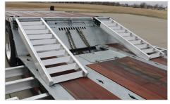
60" or 44" Aluminum Ladder Ramps for Safe Easy Transition to Rear Deck
