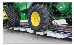
RUST FREE Aluminum Pullouts to 13' Width (7,000 lb Capacity Each on 835) (10,000 lb Capacity Each on 840)
