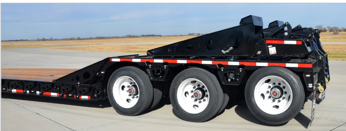
Pin-On Beaver tail, Hydraulic Flip (Pin-On Attachment to Flip Axle Brackets) – Hydraulic Brackets Required Heavy Duty Ramps – Optional Hydraulic Raise/Lower with Either Beaver tail Option
