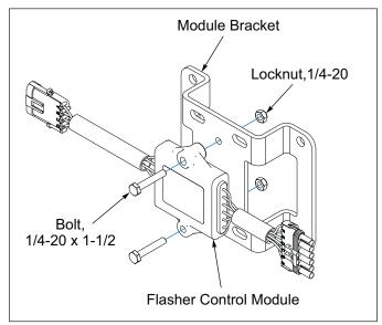
Figure 2-16: Flasher Control Module and Bracket
