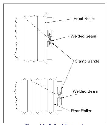
Figure 4-3: Roller Adjustment
