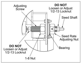
Figure 4-6: Seed Box Seed Rate Adjustment
