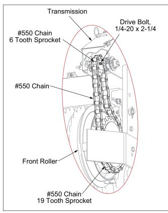
Figure 3-12: Transmission Drive Bolt
