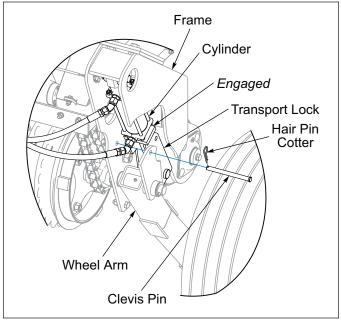
Figure 3-6: Transport Lock Engaged
