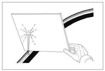
Figure 3-8: Hydraulic Leak Detection
