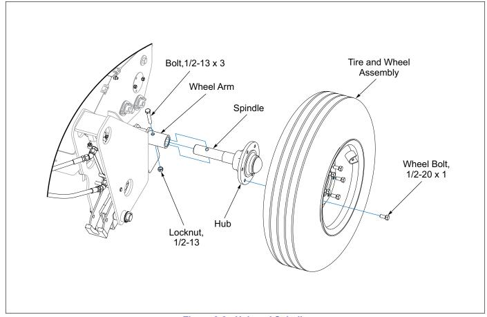
Figure 2-8: Hub and Spindle
