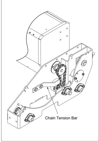
Figure 2-21: Chain Tension Bar
