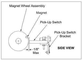
Figure 2-19: Pick-Up Switch Detail
