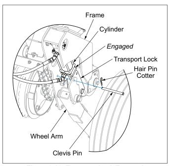
Figure 2-12: Transport Lock Engaged
