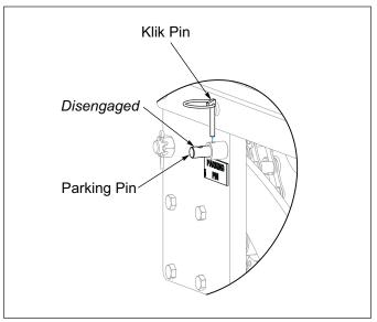
Figure 3-3: Parking Pin Disengaged
