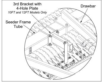
Figure 2-27: 3rd Bracket Placement - 10' & 12'
