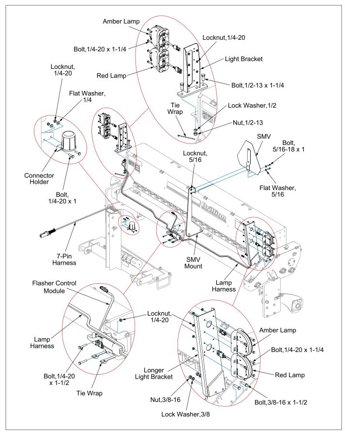
Figure 2-15: Warning Lamp Installation, 8FT 3-PT
