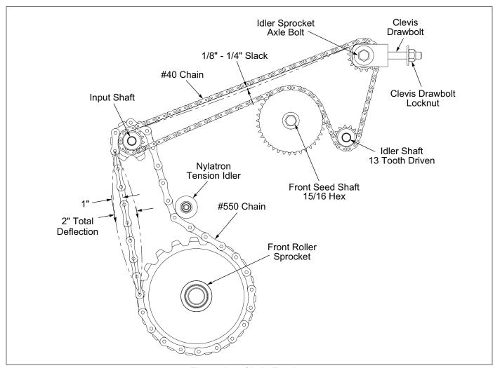
Figure 4-5: Chain Tension
