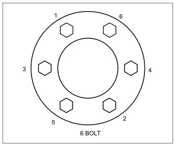
Figure 2-7: Tightening Sequence
