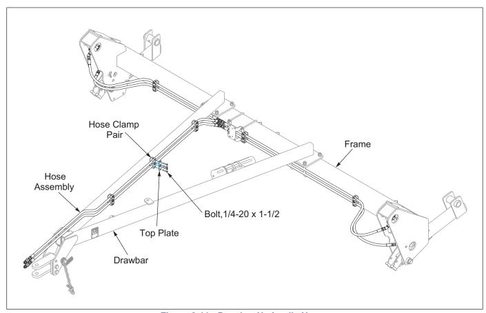
Figure 2-11: Drawbar Hydraulic Hoses
