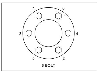
Figure 4-1: Tightening Sequence
