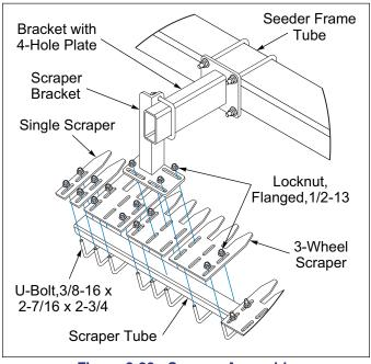
Figure 2-29: Scraper Assembly
