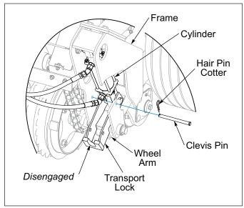
Figure 3-7: Transport Lock Disengaged
