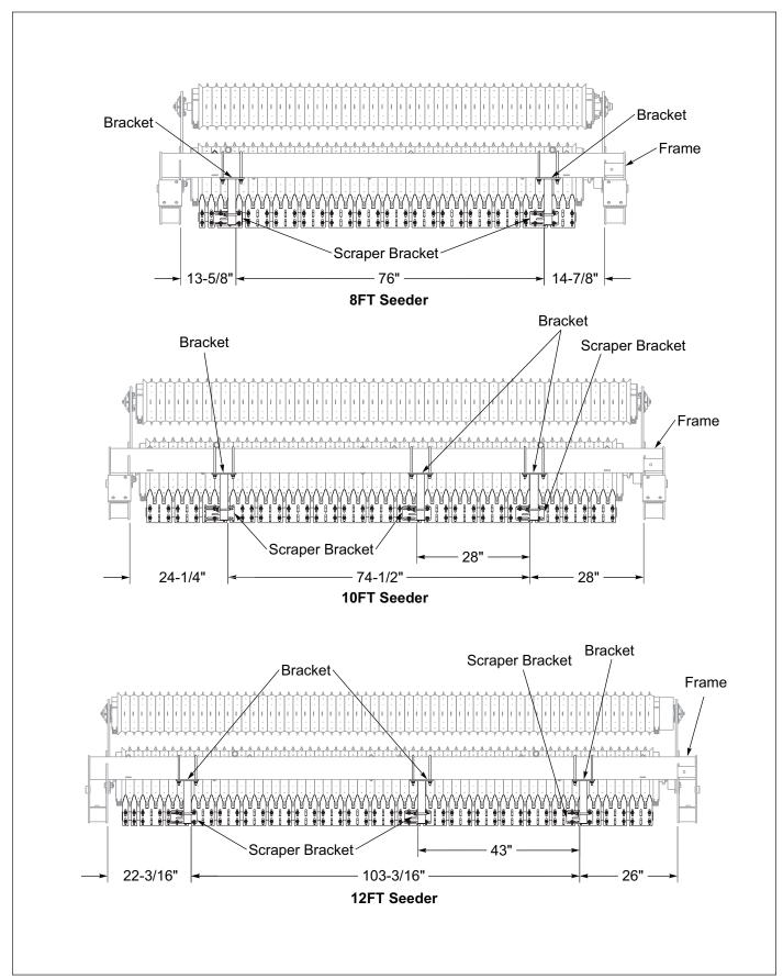
Figure 2-30: Scraper Mounting Dimensions - Pull-Type
