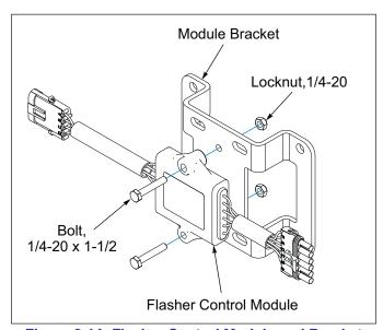
Figure 2-14: Flasher Control Module and Bracket
