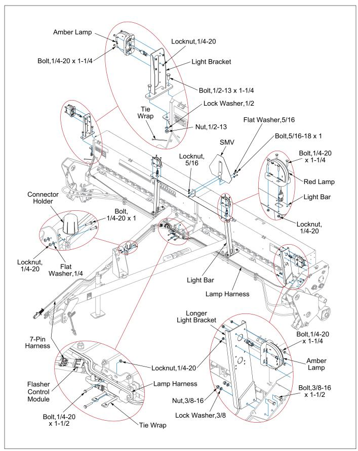
Figure 2-17: Warning Lamp Installation, 12FT Drawbar
