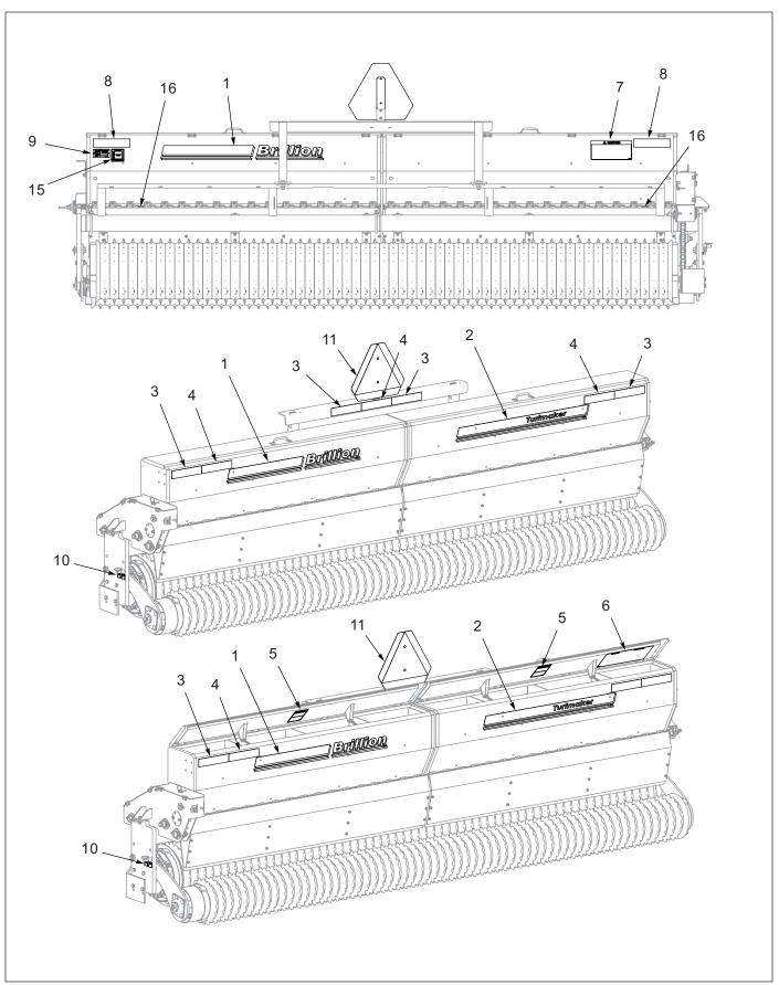
Figure 1-3: Decal Placement, 12FT Model
