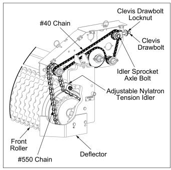
Figure 4-4: Loosen Idler Bolt
