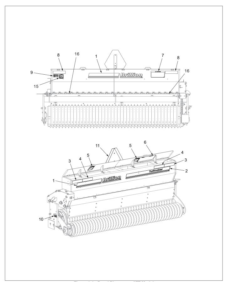
Figure 1-1: Decal Placement, 8FT Model
