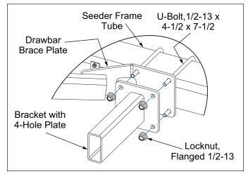
Figure 2-26: 12FT Drawbar with Braces
