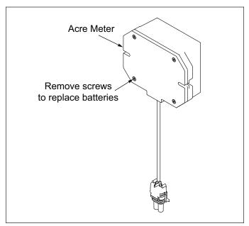
Figure 3-16: Battery Replacement
