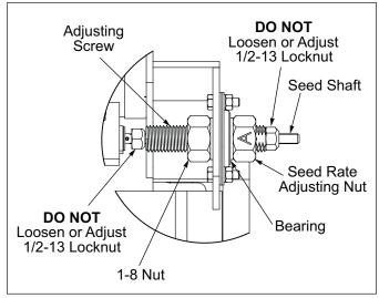
Figure 3-10: Seed Box Seed Rate Adjustment
