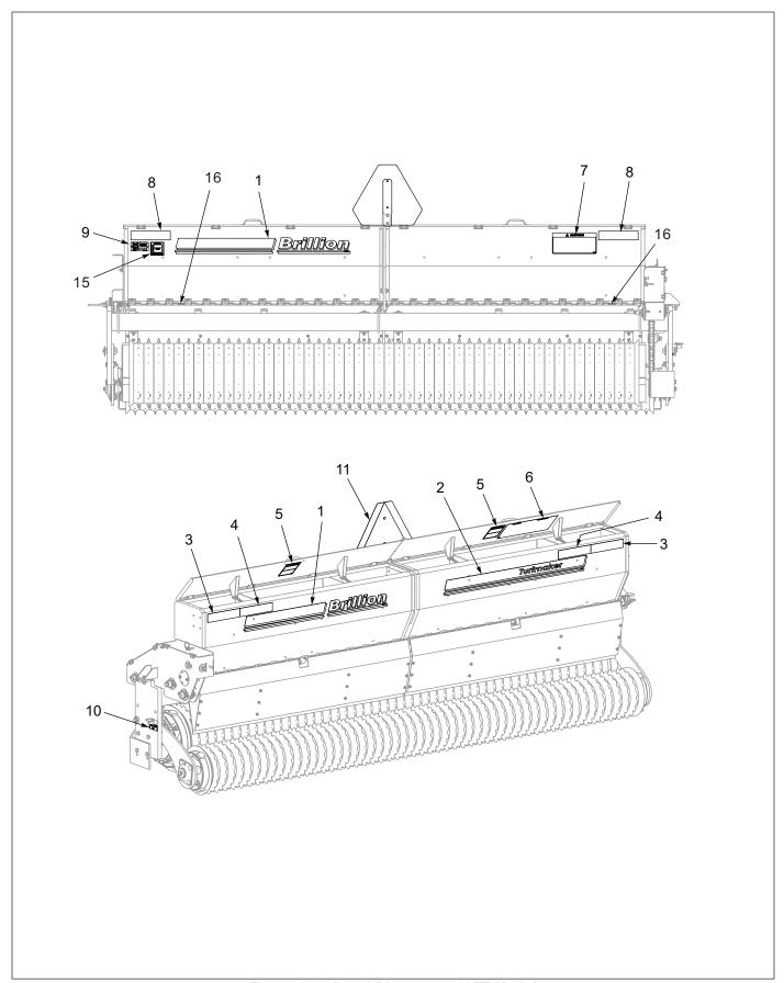
Figure 1-2: Decal Placement, 10FT Model
