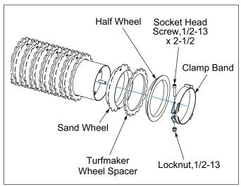
Figure 2-36: Turfmaker Sprockets
