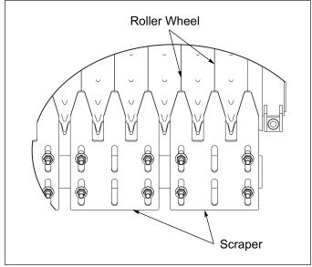
Figure 4-10: Scraper Alignment
