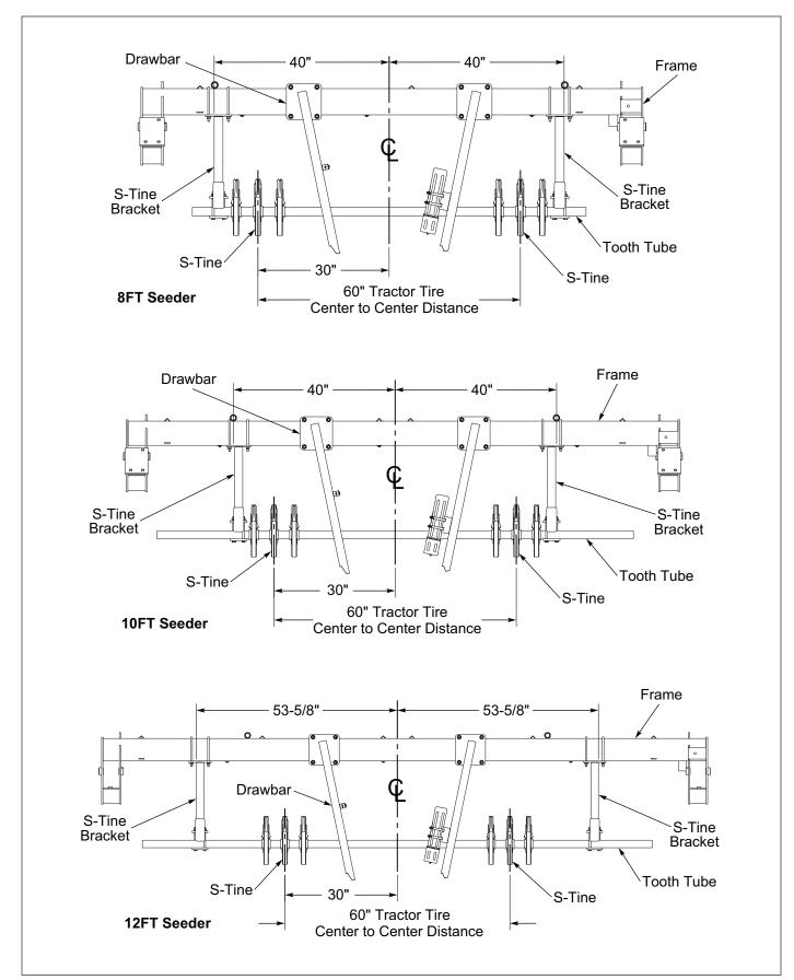
Figure 2-34: S-Tine Mounting Dimensions
