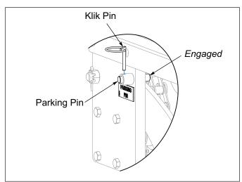
Figure 2-3: Parking Pin Engaged
