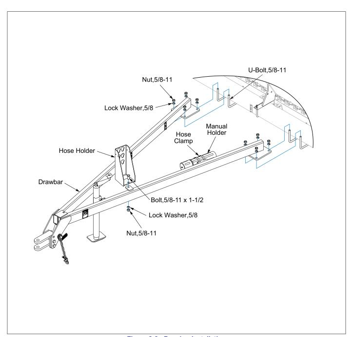
Figure 2-6: Drawbar Installation
