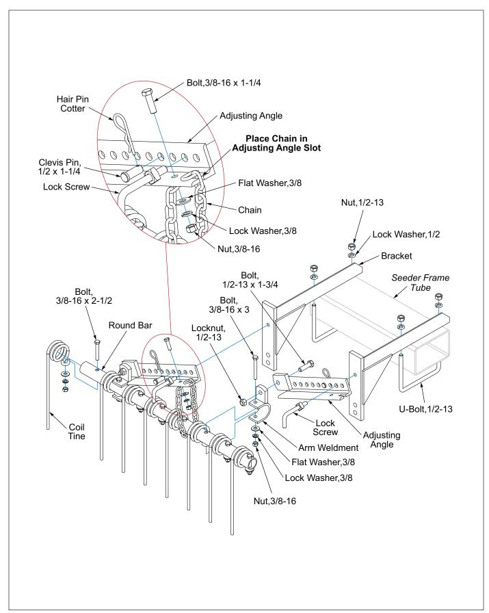
Figure 2-35: Coil Tine Track Remover - Optional
