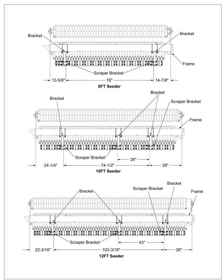
Figure 2-31: Scraper Mounting Dimensions - 3PT Hitch
