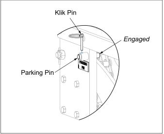
Figure 3-4: Parking Pin Engaged
