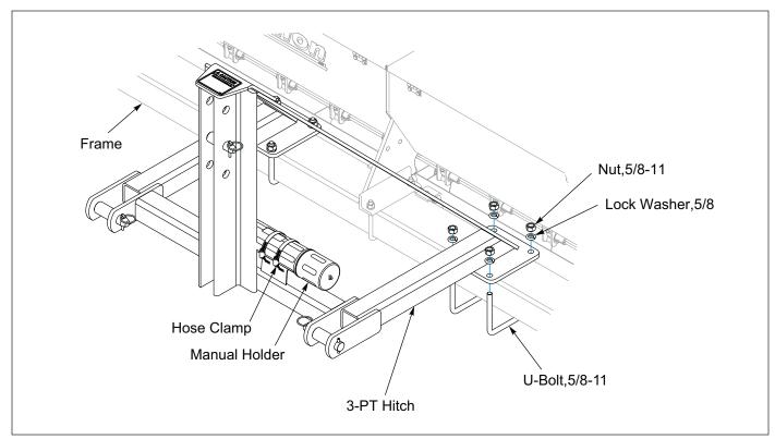
Figure 2-5: Attach 3-PT Hitch
