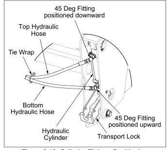
Figure 2-10: Cylinder Fittings Positioning
