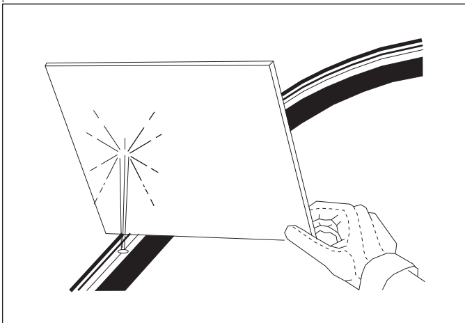
Figure 4-3: Hydraulic Leak Detection
