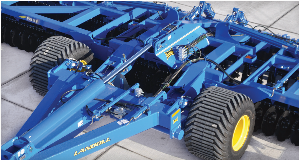
Compound Blade Arm – 17° Cutting Angle with Tilted Blade Position
