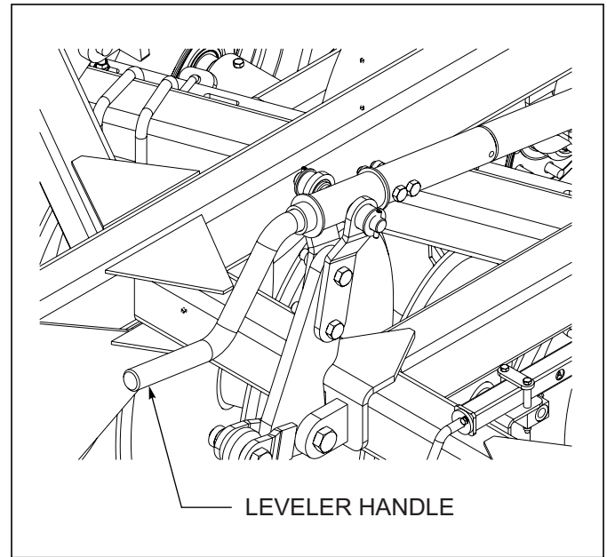
Figure 4-7: Manual Leveler Adjustment
