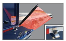
Spring Mounted Warning Flags with Holders at the Front, Drop and Rear Area
