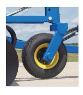
They are standard on all 7500 Series VTs. The wheel pivots on maintenance-free polymer bushings and are equipped with 6-bolt double-lip sealed hubs. An adjusting wrench comes with each unit and stores on the frame.
