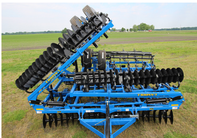
The 35' and 40' Tilloll features a stack fold system offering a transport height of 13' 0" (35') and 13' 9" (40') and transport width of 17' 9".
