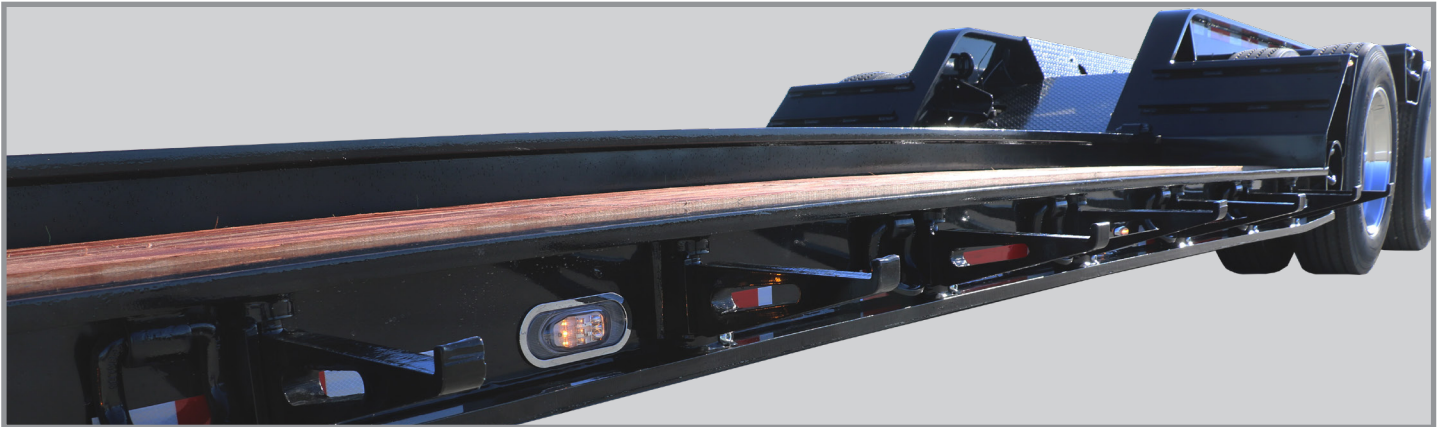
• Drop Side Swingout Outriggers on 24" Centers
