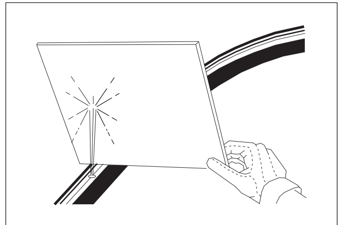
Figure 2-45: Hydraulic Leak Detection
